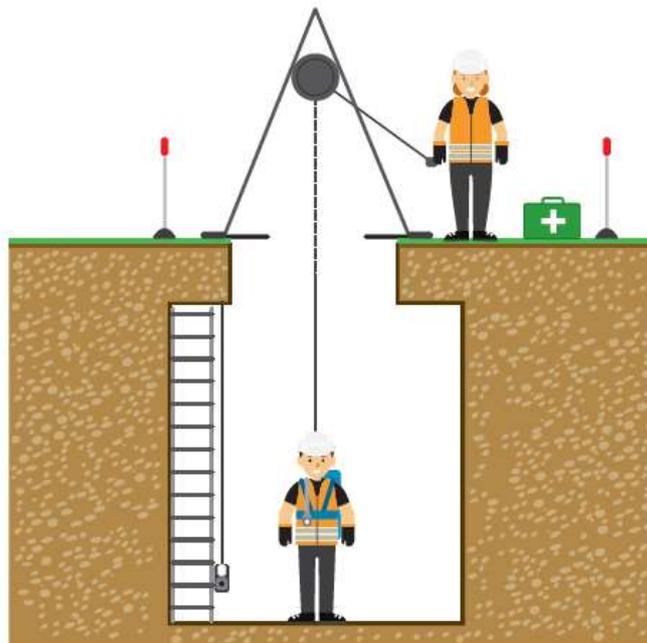
NC3 when it is not possible to have persons permanently attached to a safety line. Usually it will be a team entry which moves away from the entry point e.g. person entry sewers, utility service subway tunnels, aqueducts and complex wet wells. Working without an attached rescue line and includes working away from the point of entry but on an unobstructed horizontal plane.
