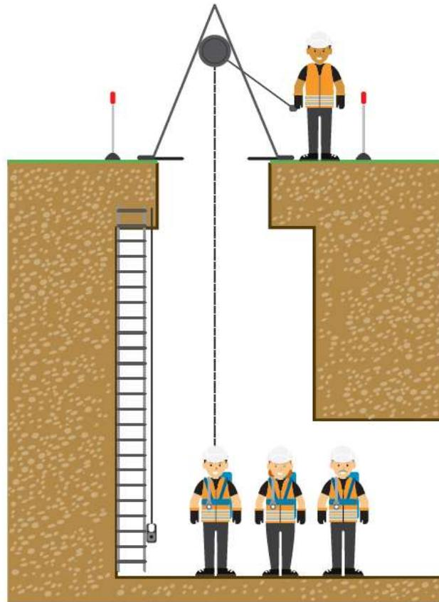
NC4 Complex access and egress that do not meet any of the classifications above or involving complex operations which introduce additional risks and require specific controls and rescue arrangements e.g. mechanical hazards, physical complexity of system introduced hazards, enhanced specific intrinsic hazards.
