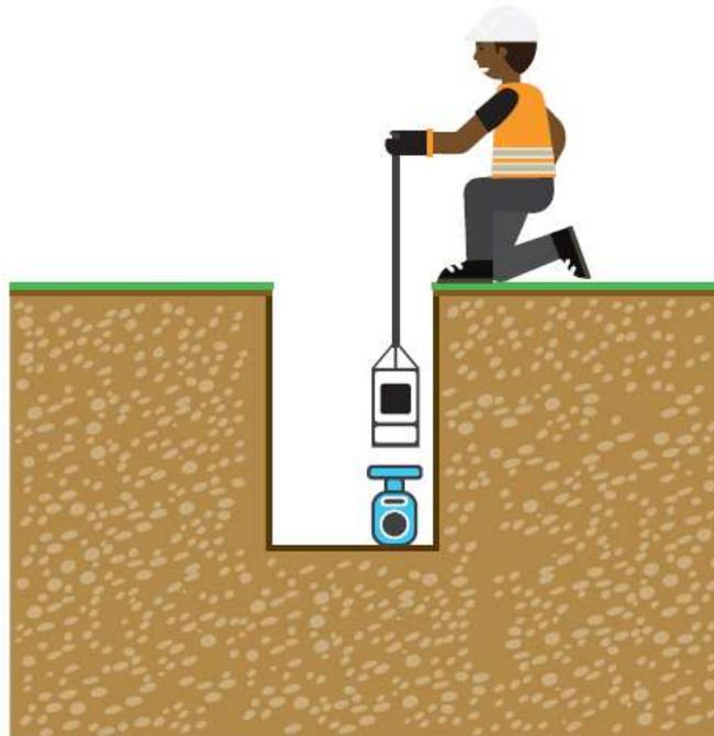
**NC2** Vertical direct unobstructed access with continuous attachment to a person riding hoist or similar mechanical rescue device.
