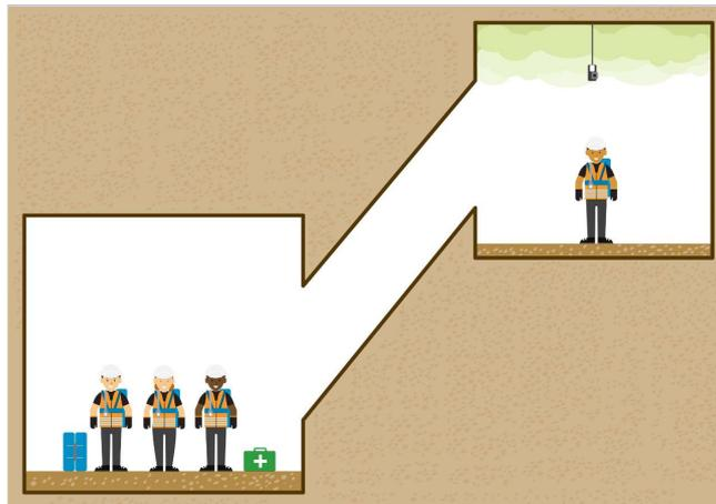
It should be remembered that not all confined spaces are vertical entry spaces. Some are horizontal entry (e.g. rooms or spaces with gas storage or combustion plant), others have vertical upward entry (e.g. roof spaces where methane or hydrogen could accumulate). Specific atmospheric analysis, access arrangements and rescue plans must be devised for each such space encountered.
